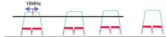
Two adjacent channels need to be clustered in one filter cavity otherwise processors such as the TSMP ,range TSMP-TV-TVDTQ have to be used as shown in the following pages.
