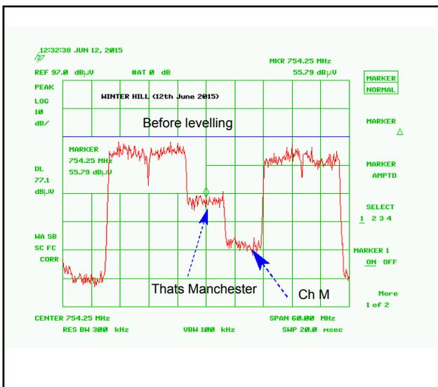
This may not be needed on small systems as using a larger amplifier could accommodate the different levels without overloading ,but on medium to large systems or fibre networks ,levelling is very important .
