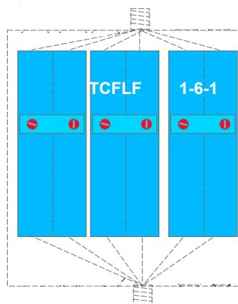
One input, one output used for levelling off air multiplexes from a single antenna, use two input connectors for separate antenna inputs, extra cost £2.90 each extra input.
